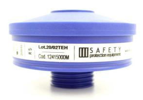
The 100 P3 R filter, with the standard thread connector (EN148-1, RD 40-1/7") can be used with the full face gas masks type SGE150, SGE 400/3 and SGE 400/3 BB, or equivalent and with the APA (Aria Protection adaptor) assembled on Ocean Reef snorkelling masks (Aria and UNO series). This filter protects against aerosols, particles, mist, fumes and dust.
